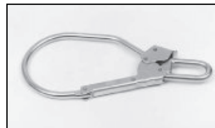
3034 (Option B) Large Locking Rebar Hook 15/16" eye (I.D.) 3 11/32" opening 13" length Rated to 3968 lbs. (Only to be used on shock absorbing style lanyards)
